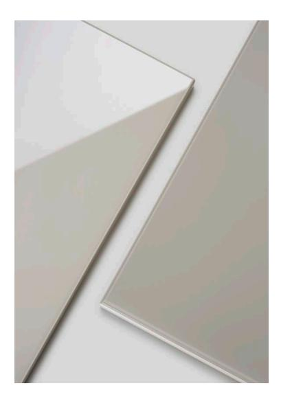
The RAUVISIO crystal acrylic surfaces are laminated onto super-refined MDF using specially formulated PUR glue in a clean room environment to ensure an optical grade reflective quality and perfectly balanced panels.
